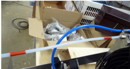
Figuur 7: Zuigslang tank 5 sec over 20 centimeter is 3 liter/uur.
