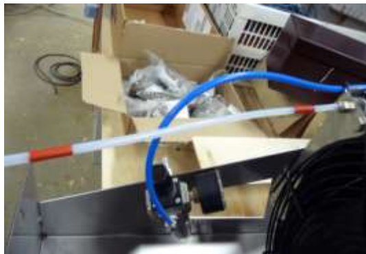
Figure 6: Suctioning hose tank 5 sec. over 20 cm is 3 litres/hour.
