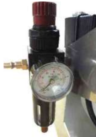
Figure.5: Pressure-reducing valve with pressure gauge
