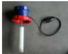
Figure 4: The stirring mechanism for the liquid supply
